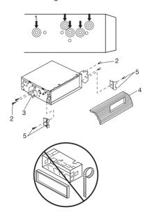
Fastening the unit to the factory radio mounting bracket.
